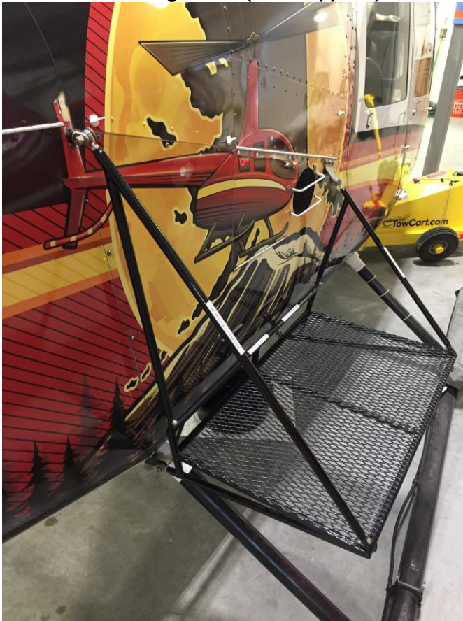
Installed Rack – Right Side (on a Clipper II) – Looking foward
